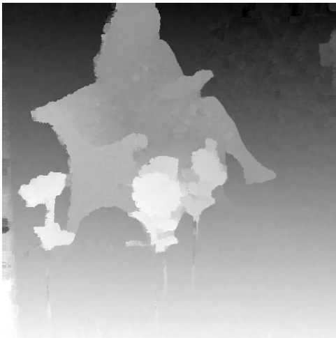
Figure 7: Stereo disparity map computed using the multiple window based parallax for a pair of frames for Region 1 in the Redcar sequence.
